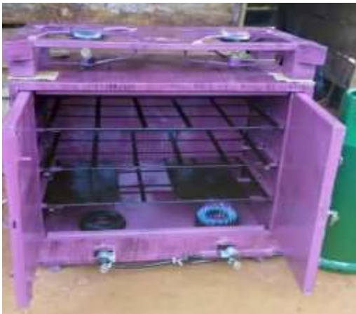
Fig. 3.4 Assembly View of the Gas oven
